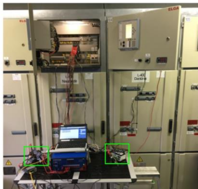
Figure 18 Test setup with EOR-3D for two feeders
